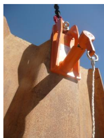
Pull the string to carry out remotely of 180° rotation of the axis.
