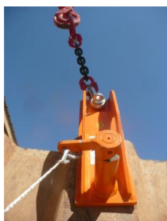
Pull the string to carry out remotely of 180° rotation of the axis.
