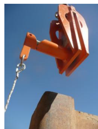
The clamp releases the sheet pile.
