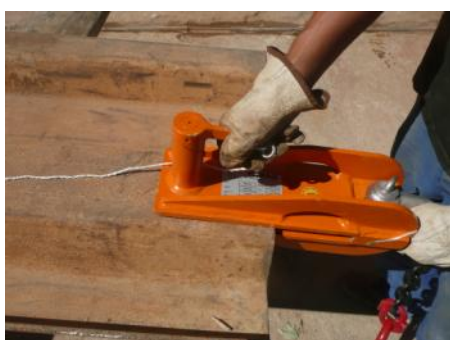
Lock the axis with a simple 180° rotation.
